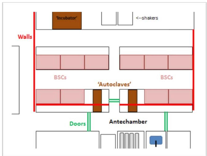
Figure 1: Conversion of Nash 304 space into mock BSL-3 laboratory.
