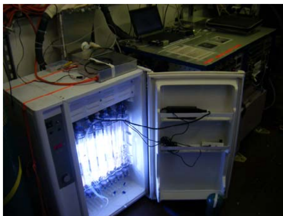
Dynamic stripping cells linked to the PTRMS for measurement of VOC metabolism in the oceans.
